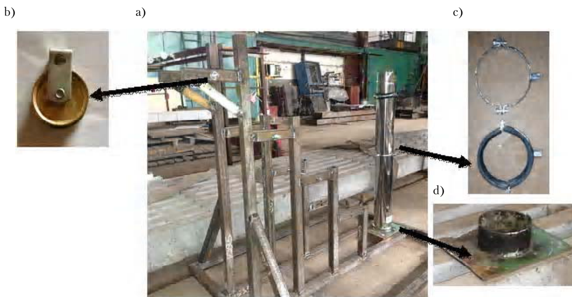
Figure 7. General view of the laboratory setup and main structural elements: a) laboratory setup with a studying model; b) roller for load transfer; c) support rings; d) support part.
