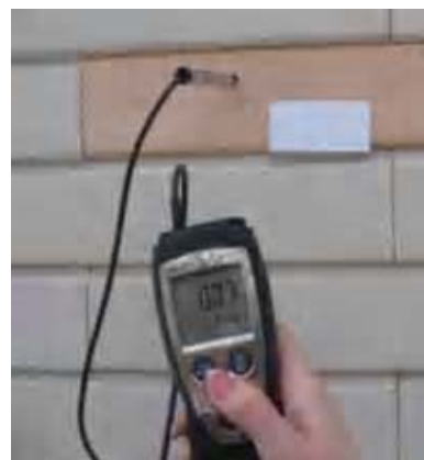
Figure 2. Use measuring devices – anemometer Testo 425.
