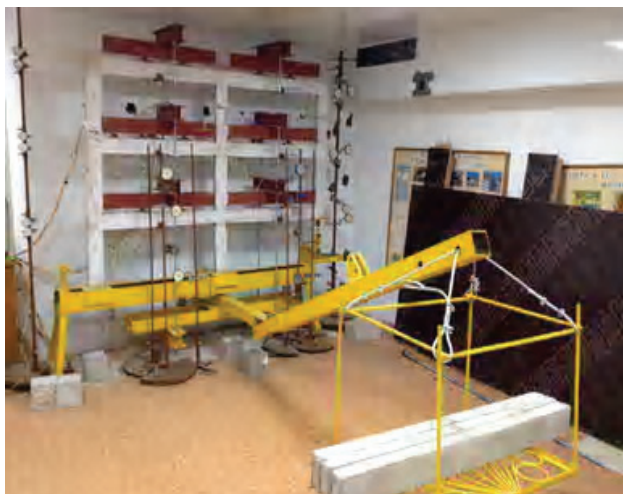
Figure 6 – A flat two-span three-story frame with a sudden shutdown of the middle or extreme pillar of the first floor.
