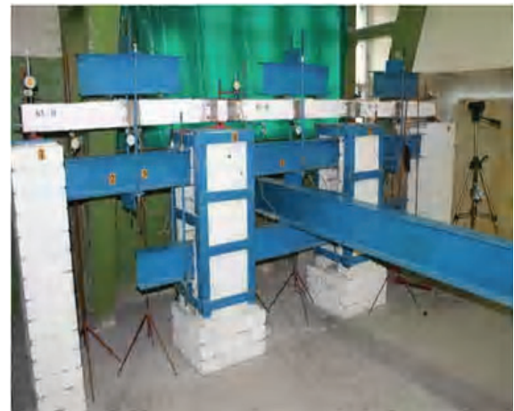
Figure 5 – Three-span beam of solid or composite section, without or with prestressing in a case of sudden disconnection of the torque coupling in the section above the support: 1 – experimental beam design; 2 – loading platform with loads; 3 – lever; 4 – switchgear; 5 – supports; 6 – over-bearing connecting part; 7 – calibrated connecting part.
